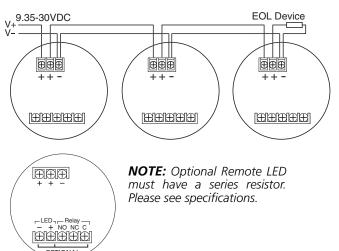
**CAUTION:** Do NOT use looped wire under terminals. Break the wire run, to provide supervision of connections
