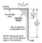
Do **NOT** locate smoke detectors at the top of peaked or gabled ceilings; the dead air space in these locations may prevent the unit from detecting smoke. Avoid areas with turbulent air flow, (near doors, fans or windows. Rapid air movement around the detector may prevent smoke from entering the unit. Do **NOT** locate detectors in areas of high humidity.
