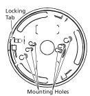
Mount backplate on standard 4" octagonal electrical box using the screws provided.
